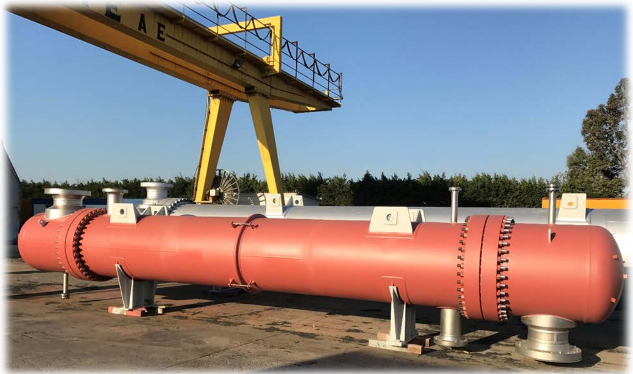
010-E-305 Feed Water Preheater
