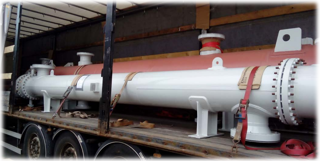
010-E-411 Natural Gas Compressor Recycle Cooler
