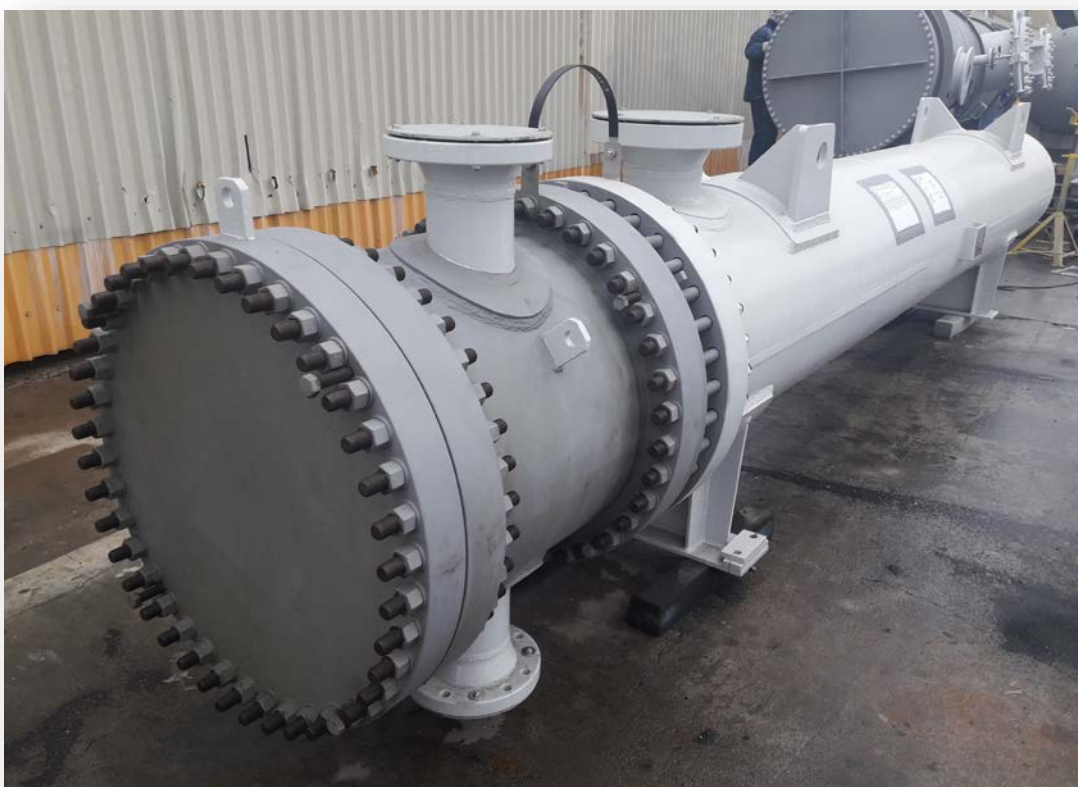
E-5005 Ethylene Cooler
