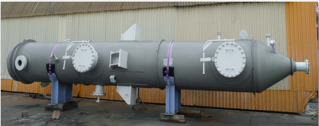
T-3001 Intermediate Treatment Scrubber
