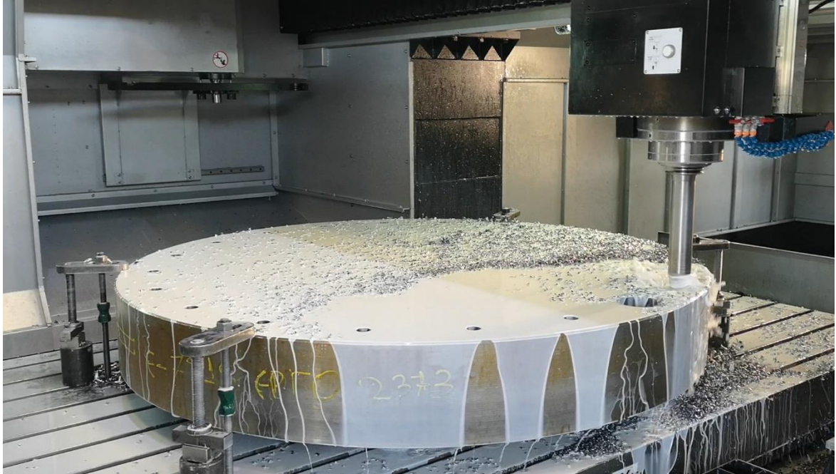
Cover Holes \Phi 106 \times 320 \text{mm} drilling (Edgecam 2018 machining software)
